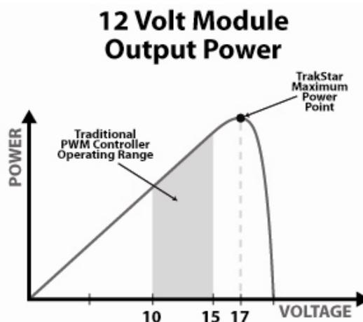
A consequence of this is: the less charged the batteries are (lower battery voltage), the more “boost” current they will receive. This is precisely the time when batteries will benefit from an increased amount of charging current.
